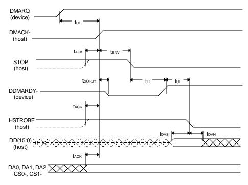
Figure 5 - 9 Initiating an Ultra DMA Data Out Burst
