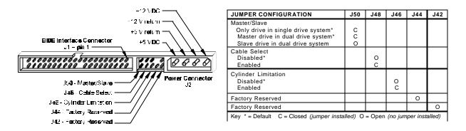
Figure 2-1 PCBA Jumper Location and Configuration
