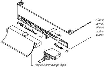
After attaching the IDE interface cable and the power cable to the Maxtor hard drive, verify that all other cables connected to other devices, the mother board or interface card(s) are correctly seated.
